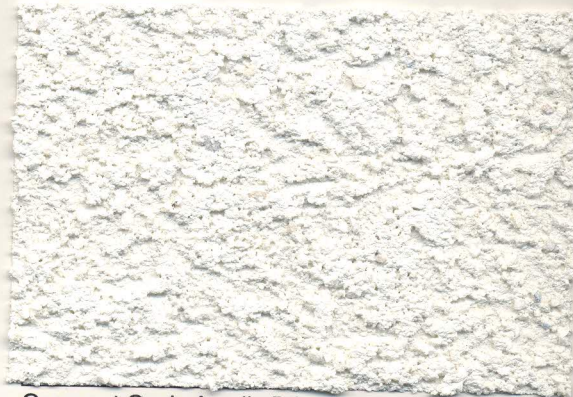
One coat Oasis Acrylic Primer One coat Oasis Flushcoat Smooth White
